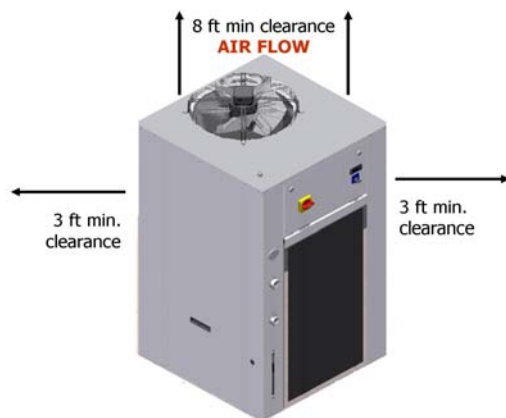
Figure 1. Minimum Installation Clearances
